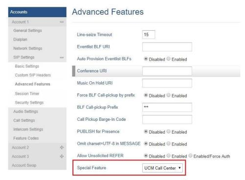
After saving and applying changes, a softkey labeled "UCM-CC" will appear on the bottom
