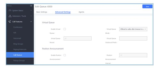
In addition to the existing basic queue functions, the Call Queue page now offers the following new features: Virtual Queue, Position Announcement, Switchboard and Call Queue Statistics.
